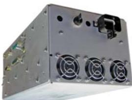
Behlman 94075 COTS VME power supply is the newest addition to Behlman's line of power supplies for UHF SATCOM terminals
