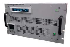
The new Behlman AFC-7003, AC Power Source/Frequency Converter is helping a major aircraft manufacturer accomplish accelerated testing of new aircraft to reduce the years needed to meet certification requirements. Converts varying frequency aircraft AC power to clean, regulated, 3-phase, 115/200 VAC at 50, 60, or 400 Hz.
