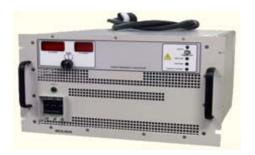
The Behlman FC5003 is an ultra-rugged COTS power supply designed to convert common 120/208 VAC, 3-phase, 60 Hz ground power to the 115/200 VAC, 3-phase 400 Hz power used by aircraft and other vehicles, as well as industrial products and systems.
