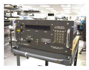
This Behlman KBT 100 AC Power Supply is one of many designed and manufactured in 1984 to support ground-based missile verification sets in ballistic missile systems. This unit has been operating successfully in rugged environments worldwide, for more than three decades. In 2015, it was received at the Behlman Factory Service Center for a tune-up.
