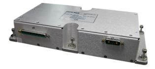
DCS1000T-1- (20, 6.25) - (20, 6.25) - (24, 16.7) is an AC-DC switch mode unit, reconfigured to support USN shipboard gun control systems. It also provides many benefits for ground and airborne systems, and industrial applications.
