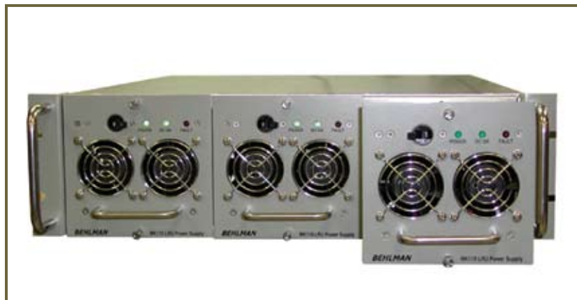
Figure 1: The Behlman MK119 Power Supply is a modified COTS modular design with three LRUs, all of which share the load. If one LRU is lost, the remaining two can support the full load while the third unit is hot-swap replaced.
