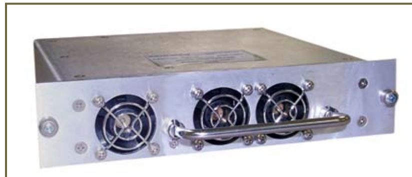
Figure 2: The Behlman 94018 COTS power supply is a switch-mode unit built for high-end applications powering work stations. It accepts a wide range of AC inputs and supplies a variety of DC outputs, supports airborne, shipboard, and mobile applications, and meets the input requirements of MIL-STD-704 and RTCA-DO160.
