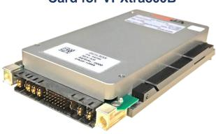
The Behlman VP*Xtra*®HU700HV COTS Hold-Up card is a rugged, highly reliable, conduction cooled, unit built for highend industrial and military applications. The VP*Xtra*® HU700HV is a 3U hold-up card expressly designed for use with Behlman's VPXtra®800B power supply to provide sufficient energy storage to hold-up 700W<sup>†</sup> of DC power for 50 msec as specified by MIL-STD-704.
