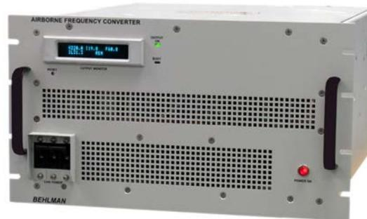
There's also a unique overload protection system that folds back voltage to maintain rated output current without waveform distortion. Units are supplied with RS-232 remote control and 28 VDC control of Output On/Off. In addition the unit has provisions for slide mounting.
