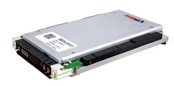
The Behlman VP*Xtra*®HU700HV COTS Hold-Up card is a rugged, highly reliable, conduction cooled, unit built for highend industrial and military applications. The VP*Xtra*® HU700HV is a 3U hold-up card expressly designed for use with Behlman's VPXtra®800B power supply to supply sufficient energy storage to hold-up 700W<sup>†</sup> of DC power for 50 msec as specified by MIL-STD-704.
