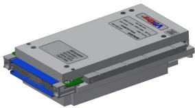
The Behlman VPXtra®HU700HV2 COTS Hold-Up card is a rugged, highly reliable, conduction cooled, unit built for highend industrial and military applications. The VPXtra® HU700HV2 is a 3U hold-up card expressly designed for use with Behlman's VPXtra®800B power supply to supply sufficient energy storage to hold-up 950W<sup>†</sup> of DC power for 80 msec as specified by MIL-STD-704.
